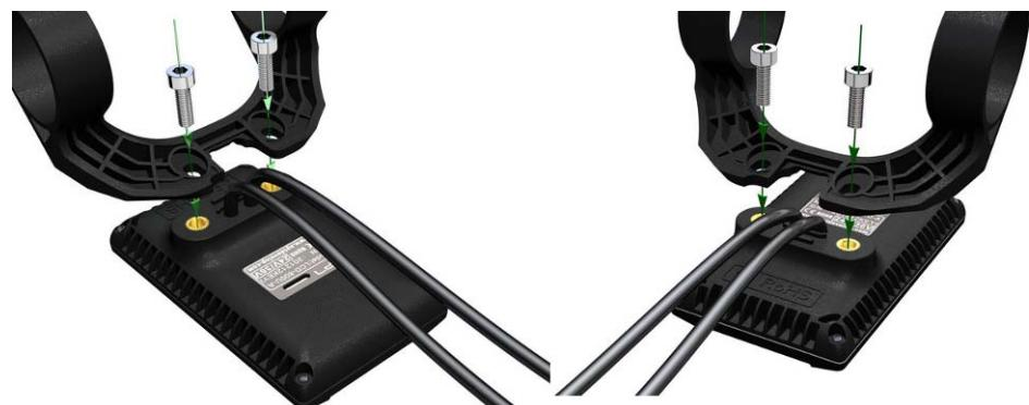
Clamps suit for 3 sizes of handlebar, 31.8mm, 25.4mm, 22.2mm, there are adaptor rings for 25.4mm and 22.2mm, adaptor ring must be assembled with the required directions, pay attention to the green arrow below.
