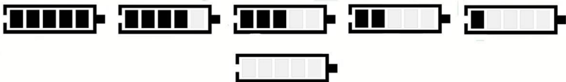
Low Voltage Flash Battery Indicator
